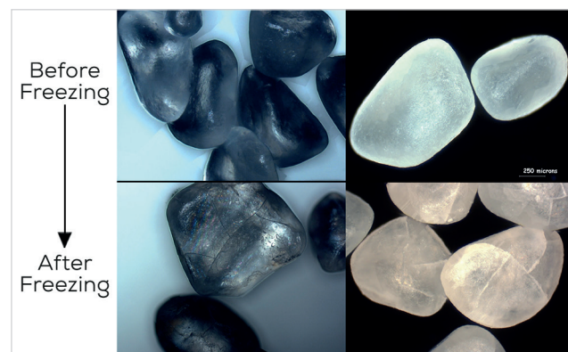
Figure 3. Freeze/thaw damage to encapsulated product.
